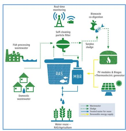
The <u>VicInAqua concept</u> is a sustainable circular ecosystem involving advanced (waste) water treatment with novel self-cleaning and antifouling membranes, innovative aquaculture with RAS, integrated water reuse, low-cost but robust real-time monitoring, energy sufficiency based on renewable sources, environmental impact assessment, awareness rising, capacity building, knowledge transfer and gender equality.
